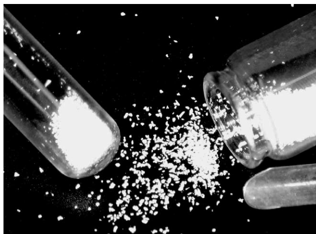
Figure 1. Polycationic Ultraresin loaded with 12 mmol/g borohydride (effective activity with 4-nitroaldehyde, rt, 16 h). The resin was sieved to a particle size of 80–170 \mu\text{m} (90–180 mesh). The reaction vessel to the left contains 1 mequiv. borohydride resin (82 mg).
